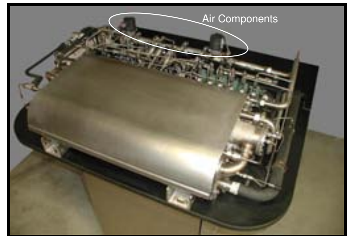
Figure 3. FPS 3A unit 3 fuel processor on test stand – 2006. Note removal of low-durability steam components, upgrade of water components, and addition of low pressure drop air system.
